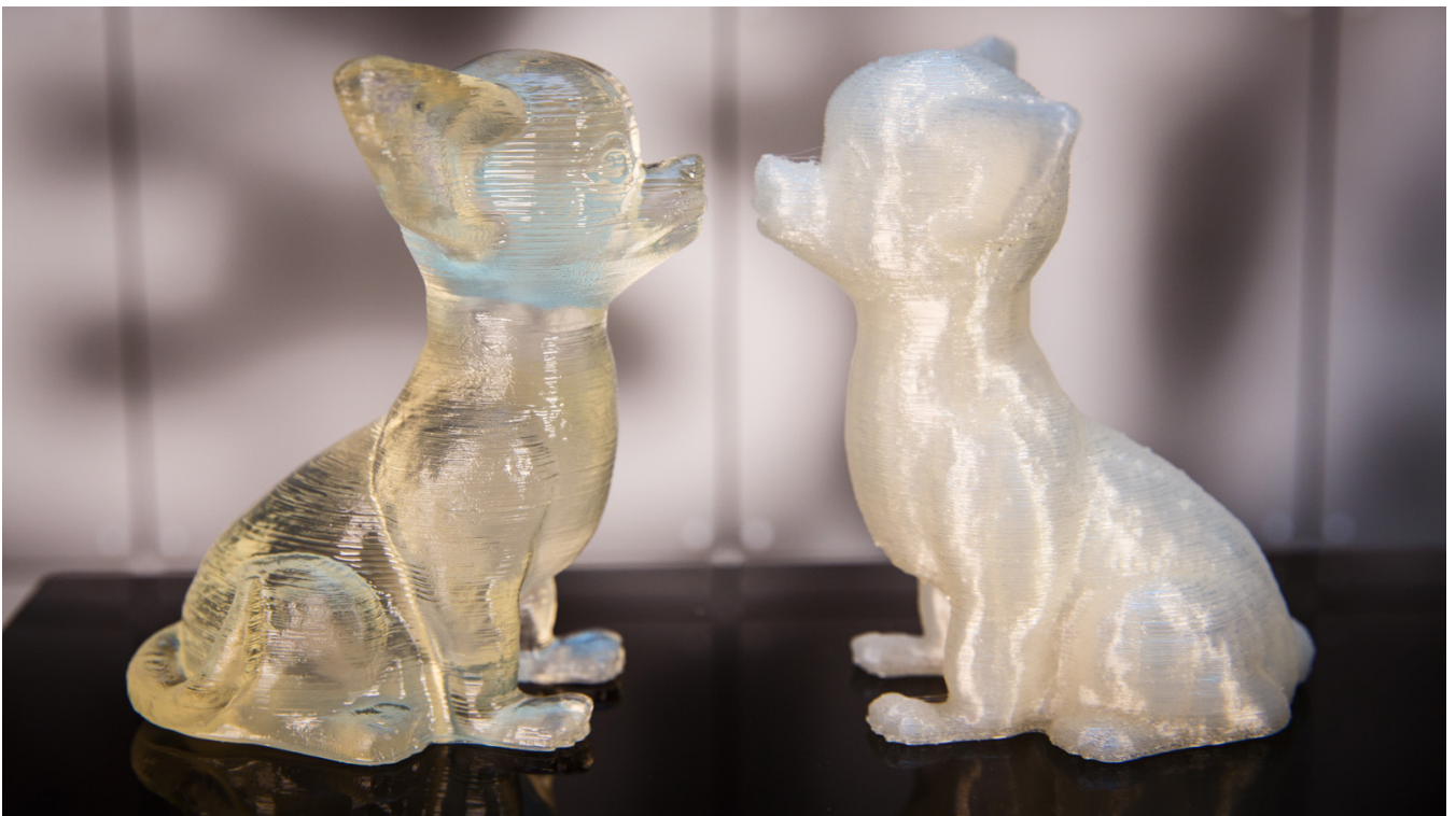
Stereolithography (SL) print on the left vs. extrusion (FFF) on the right
